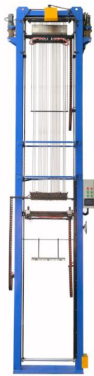
24 station filling machine (3+9+9+3 )
