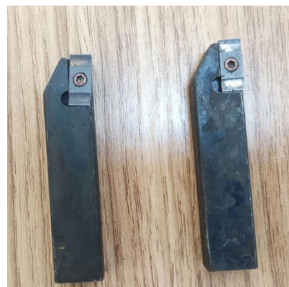
New blade for trimming Machine (not need to grind)
