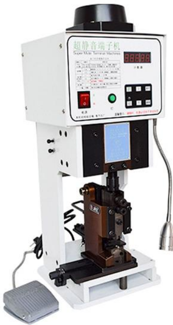
GT-TC201 Terminal Crimping Machine
