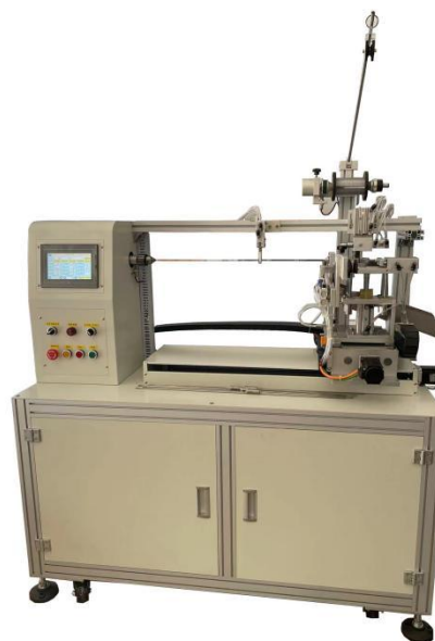
GT-DRS50 PLC winding machine with tails
