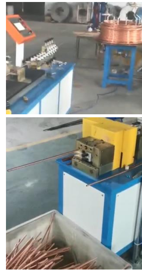
GT-ASCT19 Auto Coil Tube Straightening and Cutting Machine
