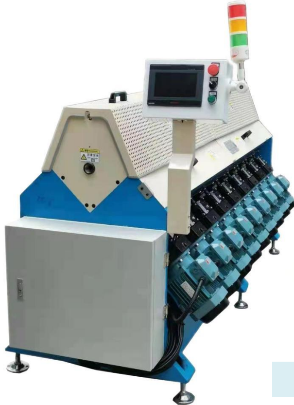
GT-JYCNC CNC Shrinking Machine
