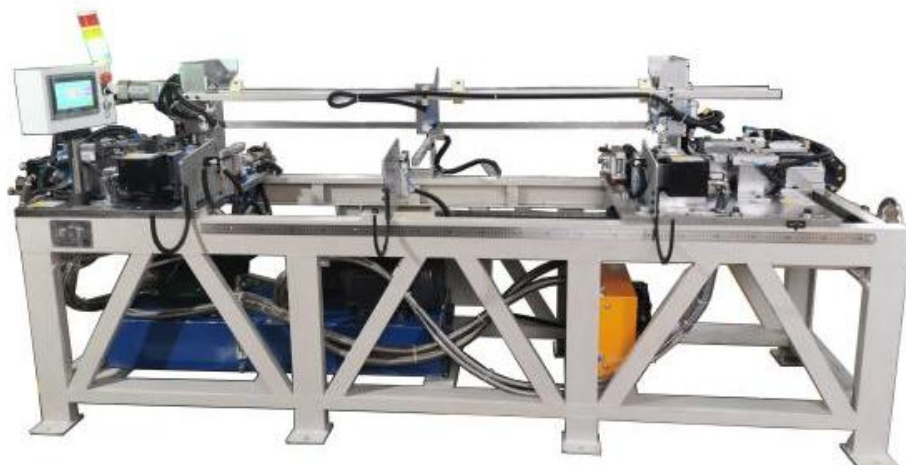
GT-LS201 Stretching Machine for Short Heaters
